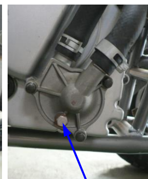
Coolant Drain Bolt
